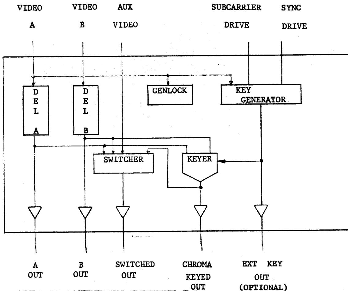
The EAB 601 / Adwar CK-3 Chroma Keyer is versatile and easy to use. It has three video inputs and four video outputs. It will either genlock or accept external drive signals. It has no color shift. A vertical interval switcher is built in for convenience. The AUX input is useful for certain non-critical switching applications. An optional External Key output is offered for use with a downstream switcher, where required (Option A).
