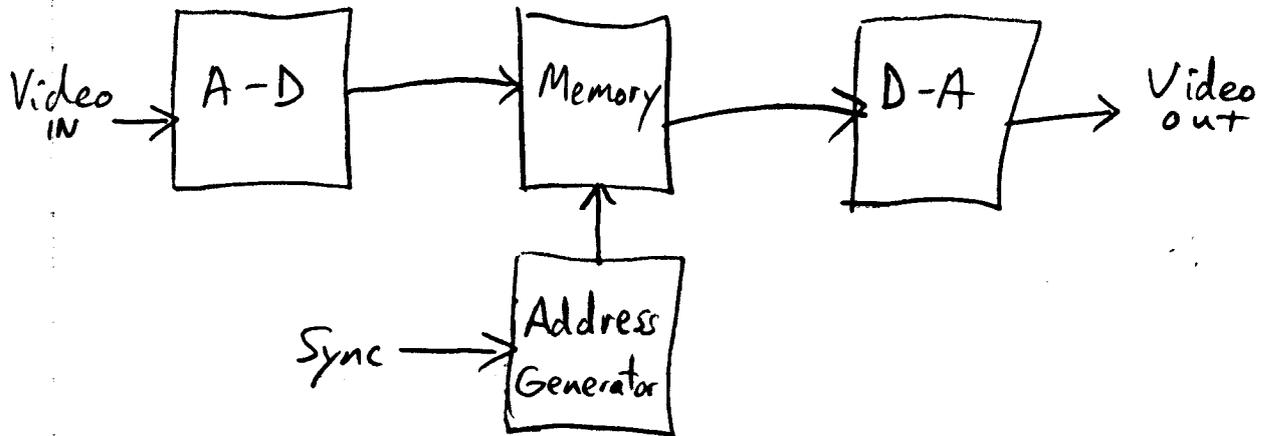
~~This Dave buffer is a simple device that can freeze a video image and display it. It is an early digital video system that converts the video image into a~~
