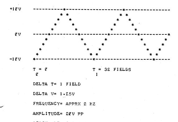
AGAIN THE TIMING INTERVAL IS SET TO 1 FIELD AND THE D/A CONVERTER SET TO QV (LINES 1-3). THE OUTSIDE LOOP (LINES 4-14) REPEATS THE WAVEFORM 1QQQ TIMES. THE FIRST INSIDE LOOP BUILDS THE POSITIVE GOING SLOPE OF THE TRIANGLE (LINES 4-6). THEN THE PEAK OF THE TRIANGLE IS FORMED (LINES 7-1Q). THE SECOND INSIDE LOOP BUILDS THE NEGATIVE SLOPE (LINES 11-13).
