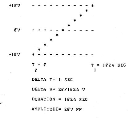
IN LINE 1 WE SET THE TIMING INTERVAL TO 60 FIELDS OR 1 SEC. WE SET THE D/A TO -10V ( LINE 2 ) AND OUTPUT THIS VALUE TO THE D/A ( LINE 3 ). NOW WE CONSTRUCT A LOOP ( LINES 4-6 ). THE LABEL L101 SETS THE TOP OF THE LOOP, THE COMMANDS TO BE REPEATED ARE ADD 100 CCTAL TO THE DATA AND OUTPUT THE NEW VALUE TO THE D/A. THIS IS REPEATED 1776 TIMES.
