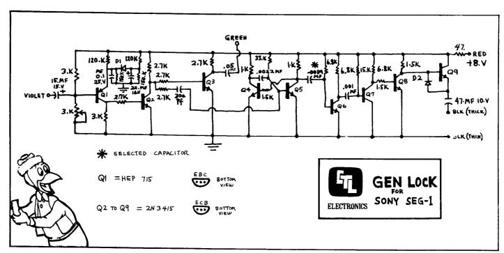
A GEN LOCK added to your Sony SEG-1 will allow you to perform wipes and fades between signals from a VTR playback and 1 to 3 live cameras. The GEN LOCK separates the sync signal from the video input and generates horizontal and vertical camera drive signals.
