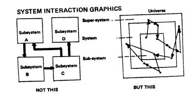
We can attempt to deal with this imbedded system by progressively modeling each one internally and then cross-connecting each with the critical "inter-imputs and out-puts" as shown.
