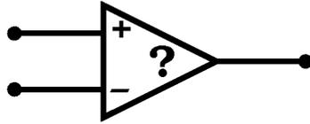
There are two inputs and one output. The inputs can be continuous voltages from, say, a scale of 0-10. The output however is allowed only two conditions: ON or OFF. The appropriate condition is determined by comparing the values of the two inputs. If the + input value is greater than the - input value, the output is ON; if the + input is the same as or less than the - input, the output is OFF. A typical circuit used for this function is the u710 integrated circuit, about the size of a dime.
