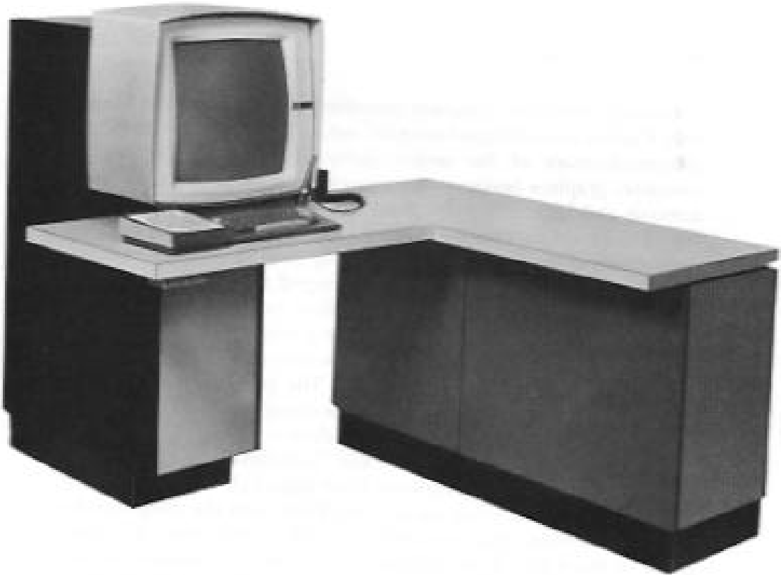
Cybernetic movie studio: The IBM 2250 Display Console with CRT, light pen, and function keyboard. Photo: IBM.
