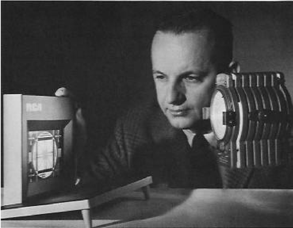
Prototype for flat, wall-size TV screens and computer visualization subsystems of the future: Dr. George Heilmeier demonstrates RCA's liquid crystal display. Photo: RCA.
