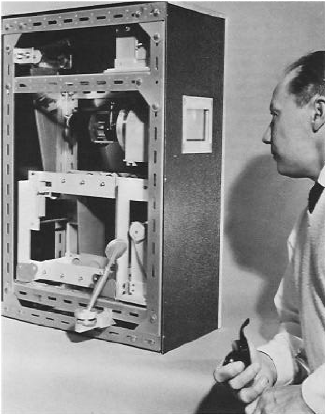
Holographic movie viewing system developed by North American Philips Corporation. Laser inside the box shines through 70mm. film as it passes viewing aperture. Photo: North American Philips Corp.
