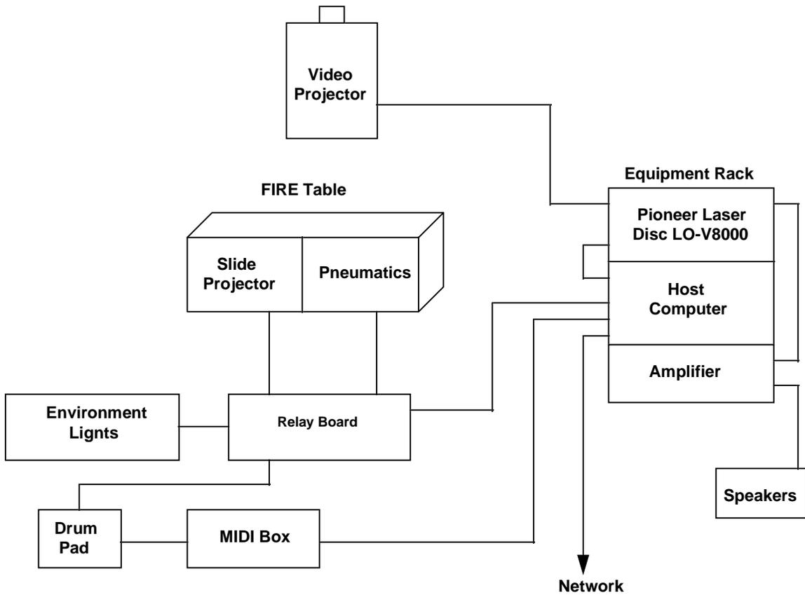
Figure II-3. FIRE System Schematic
