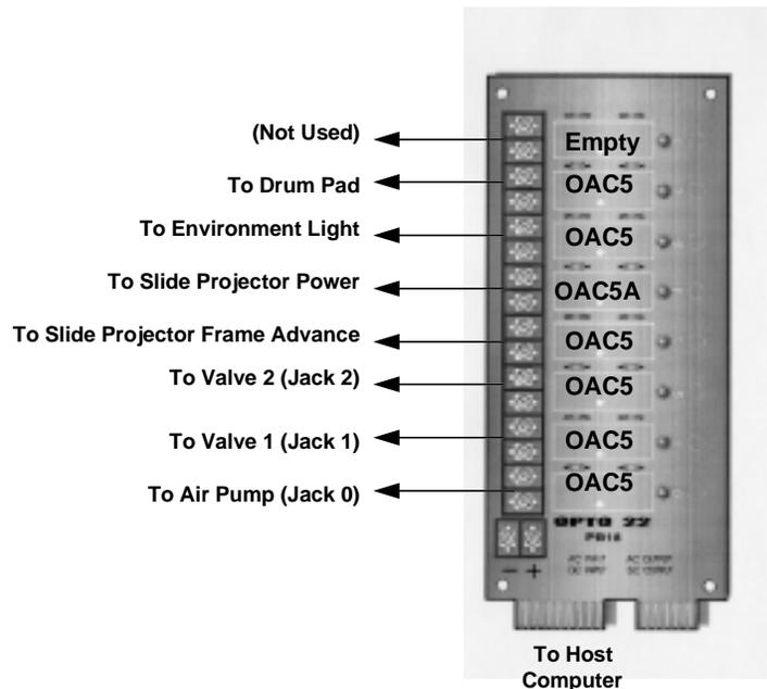
Figure II-5. Solid-State Relay Board
