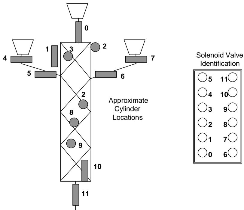
Figure IV-3. Cylinder-Valve Correspondences
