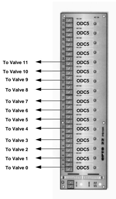
Figure IV-7. MAIDEN Solid-State Relay Board
