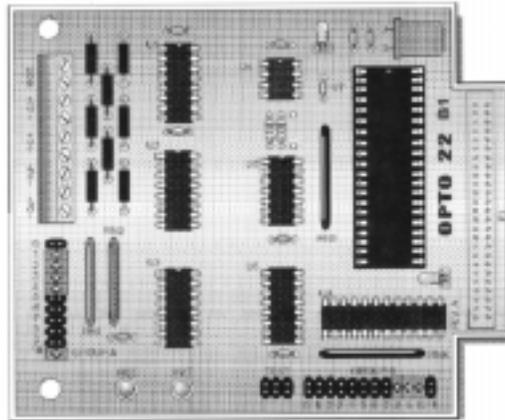
Figure IV-6. Opto22 Brainboard, Model B1
