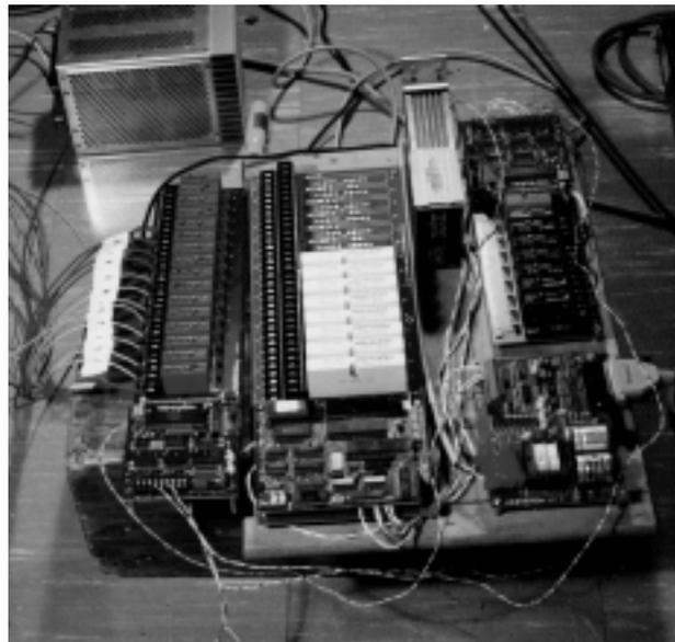
Figure IV-5. MAIDEN Solid-State Relay Board and Brainboard (left)
